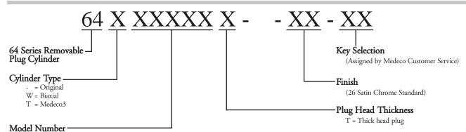
0250 = 5 pin removable plug lock, 3/4" diameter, 1 keypull
