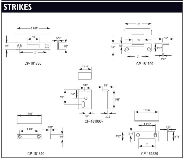
All strike plates are made of nickel plated steel
